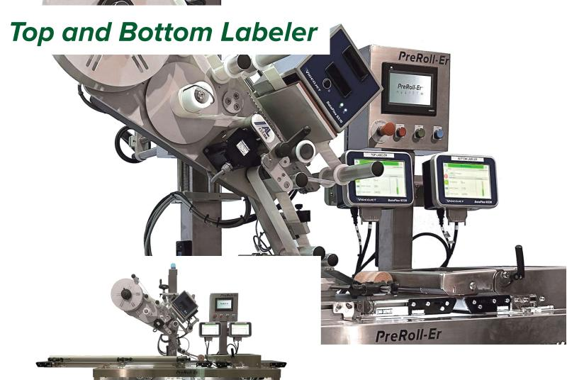
Dual head for top and bottom application simultaneously.
