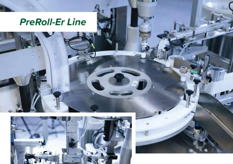
The PreRoll-Er Line is a multipurpose platform for tubes and jars with snap or twist caps.
